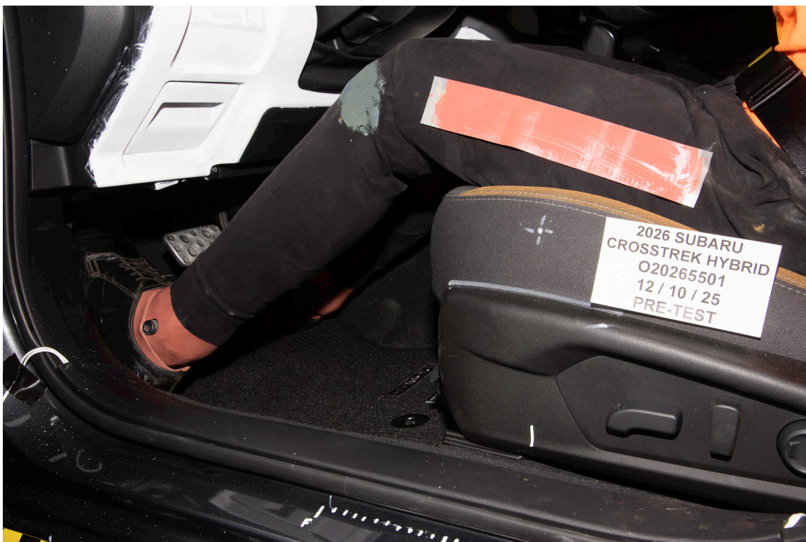
FIGURE 34. Pre-Test Placement of Driver Dummy's Feet
