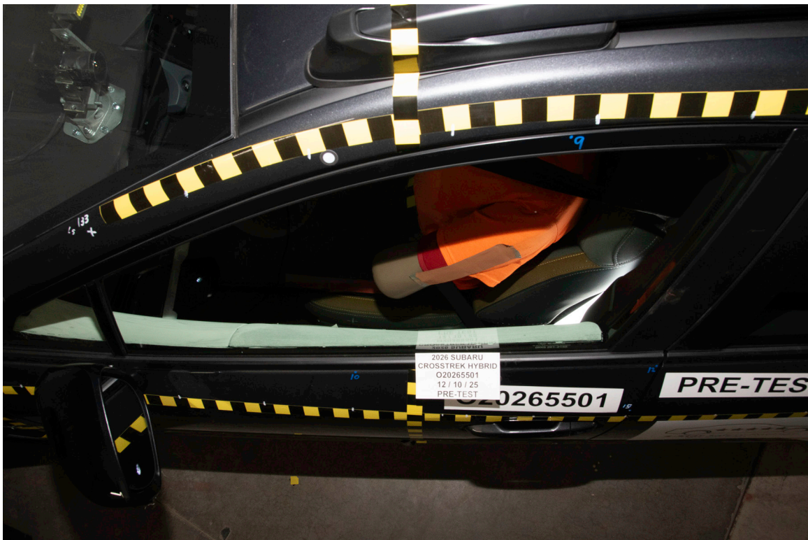
FIGURE 42. Pre-Test Driver Dummy and Door Clearance View
