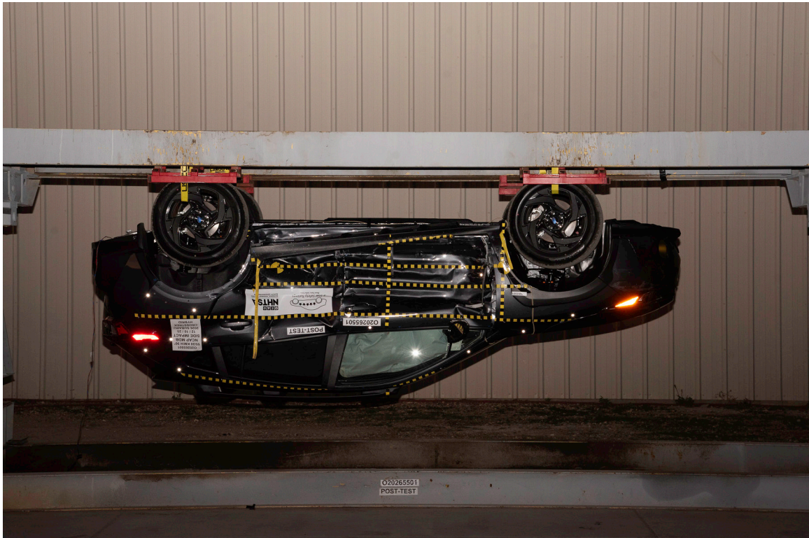
FIGURE 98. FMVSS No. 301 Static Rollover 180 Degrees
