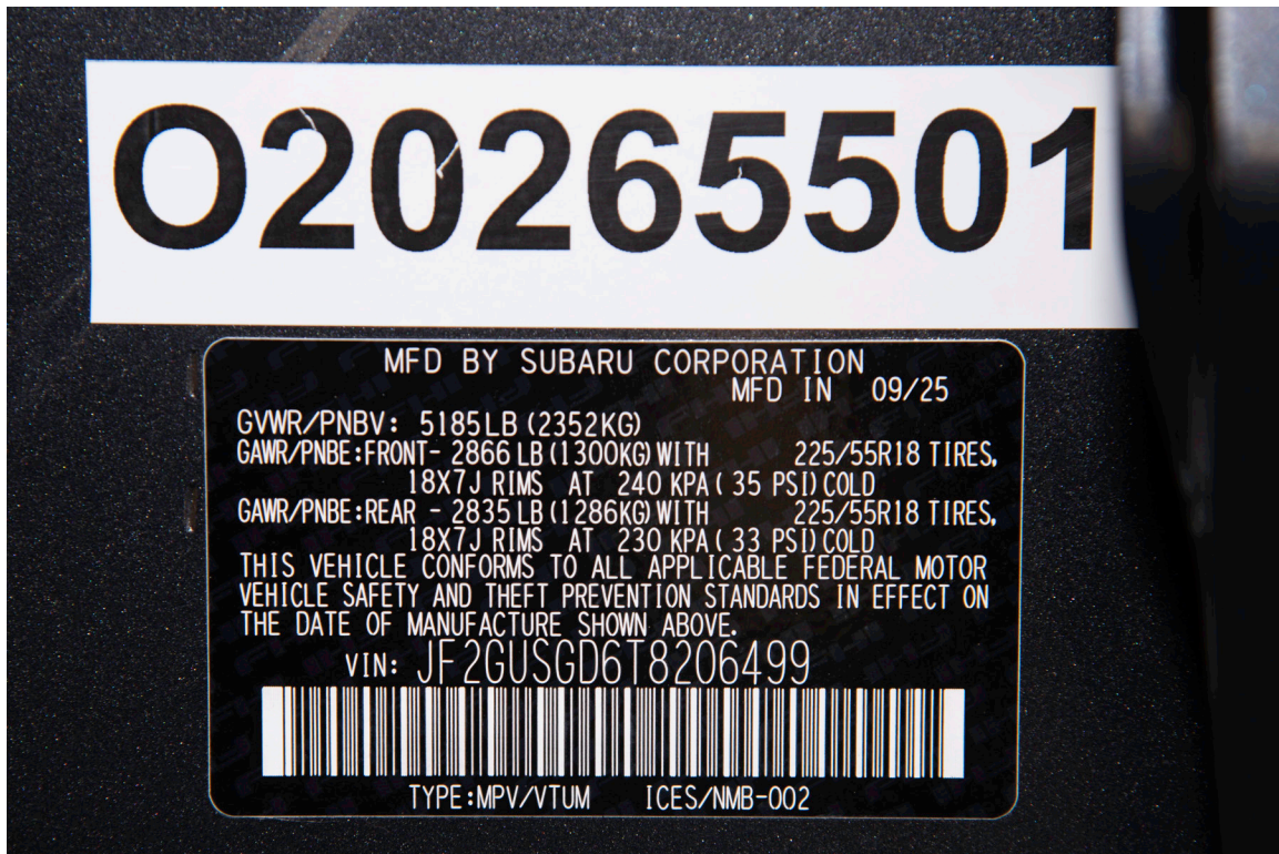
FIGURE 92. Close-Up View of Vehicle's Certification Label
