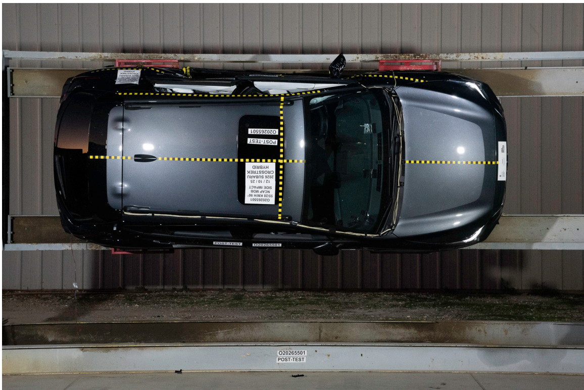
FIGURE 99. FMVSS No. 301 Static Rollover 270 Degrees
