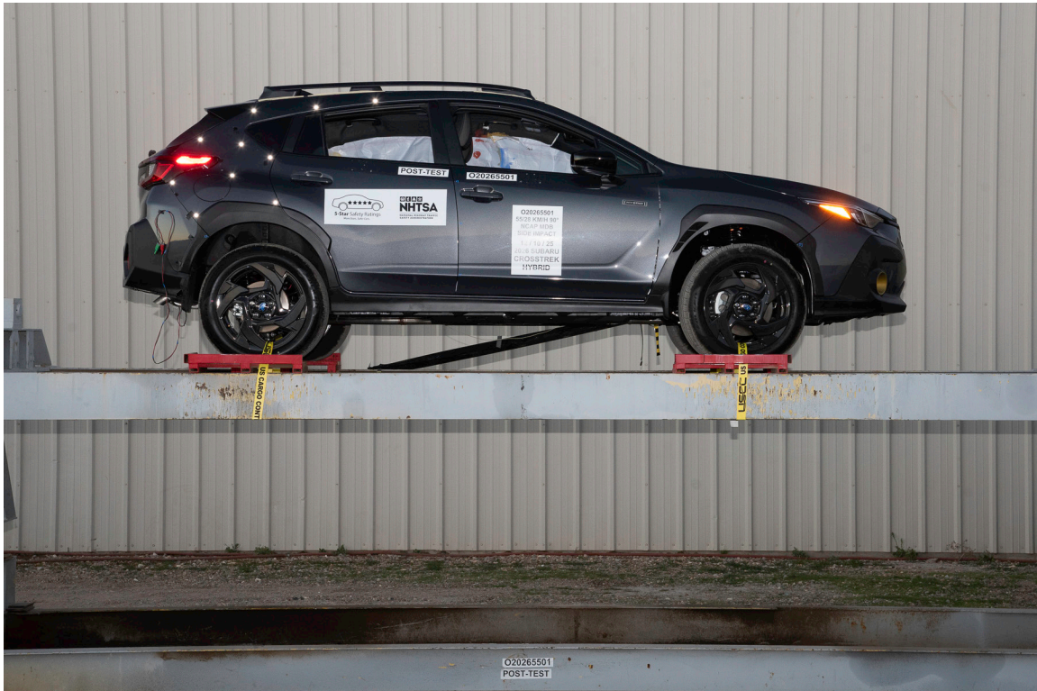
FIGURE 96. FMVSS No. 301 Static Rollover 0 Degrees
