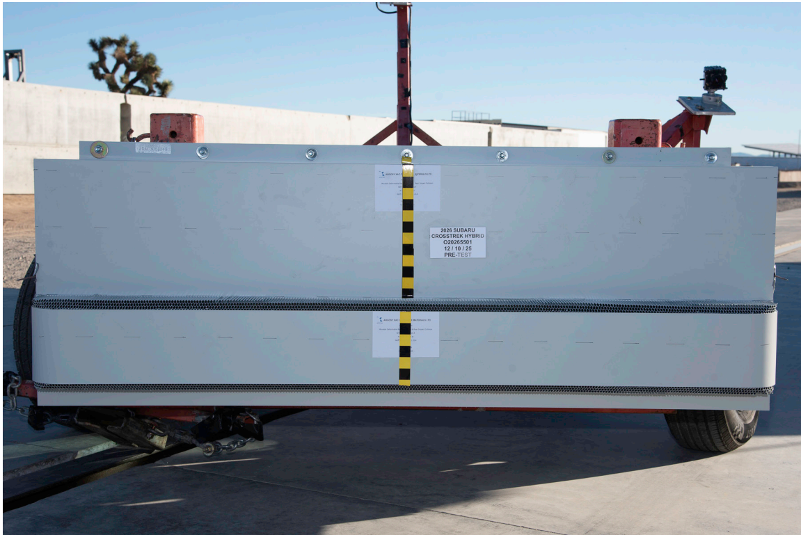
FIGURE 84. Pre-Test Front View of MDB Impactor Face
