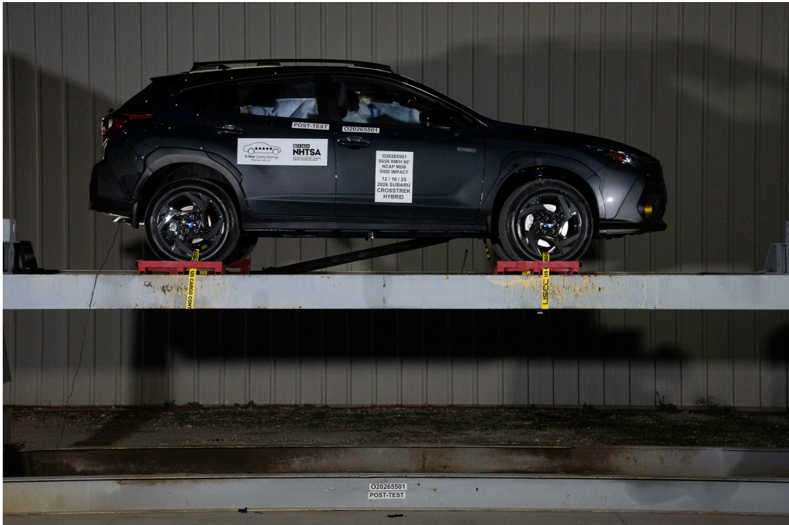
FIGURE 100. FMVSS No. 301 Static Rollover 360 Degrees
