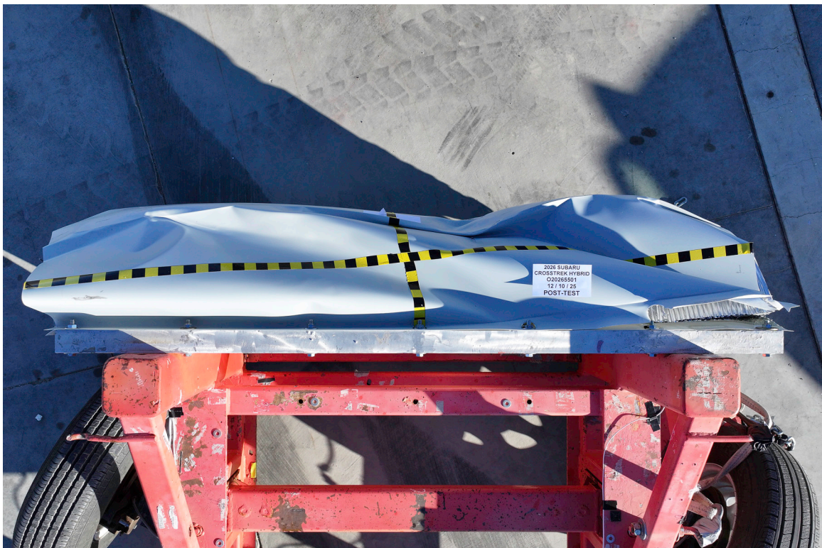
FIGURE 87. Post-Test Top View of MDB Impactor Face
