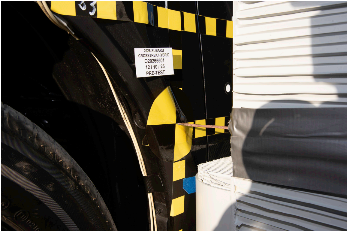
FIGURE 19. Pre-Test Close-Up View of Impact Point Target
