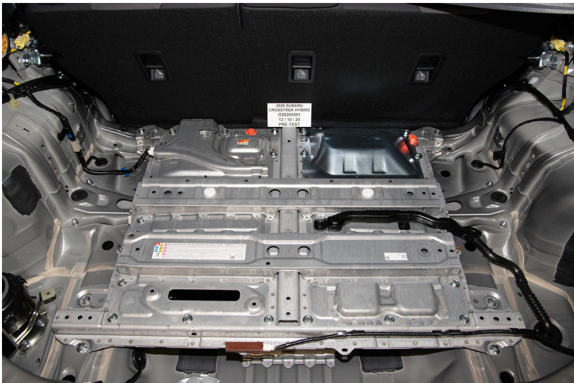
FIGURE 305-07. Pre-Impact View of Propulsion Battery
