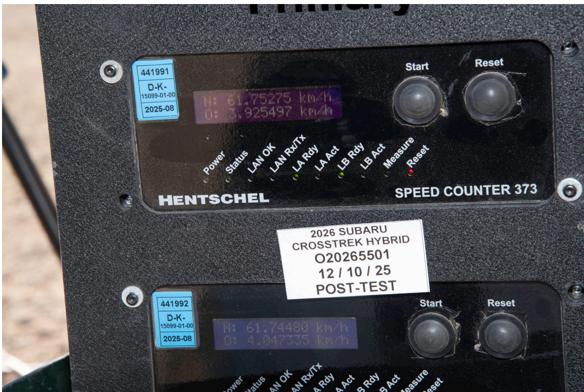
FIGURE 95. Post-Test Primary and Redundant Speed Trap Read-Out
