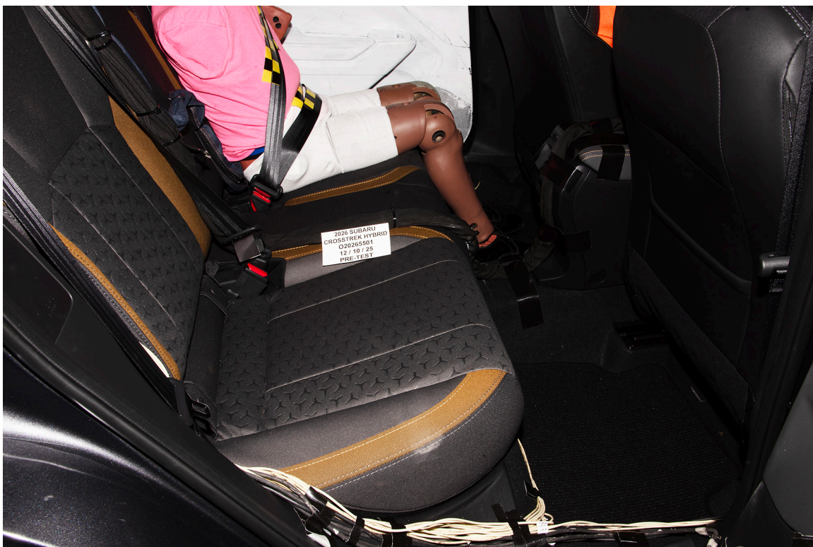
FIGURE 305-019. Pre-Impact View of the Vehicle Passenger Compartment Adjacent to Propulsion Battery
