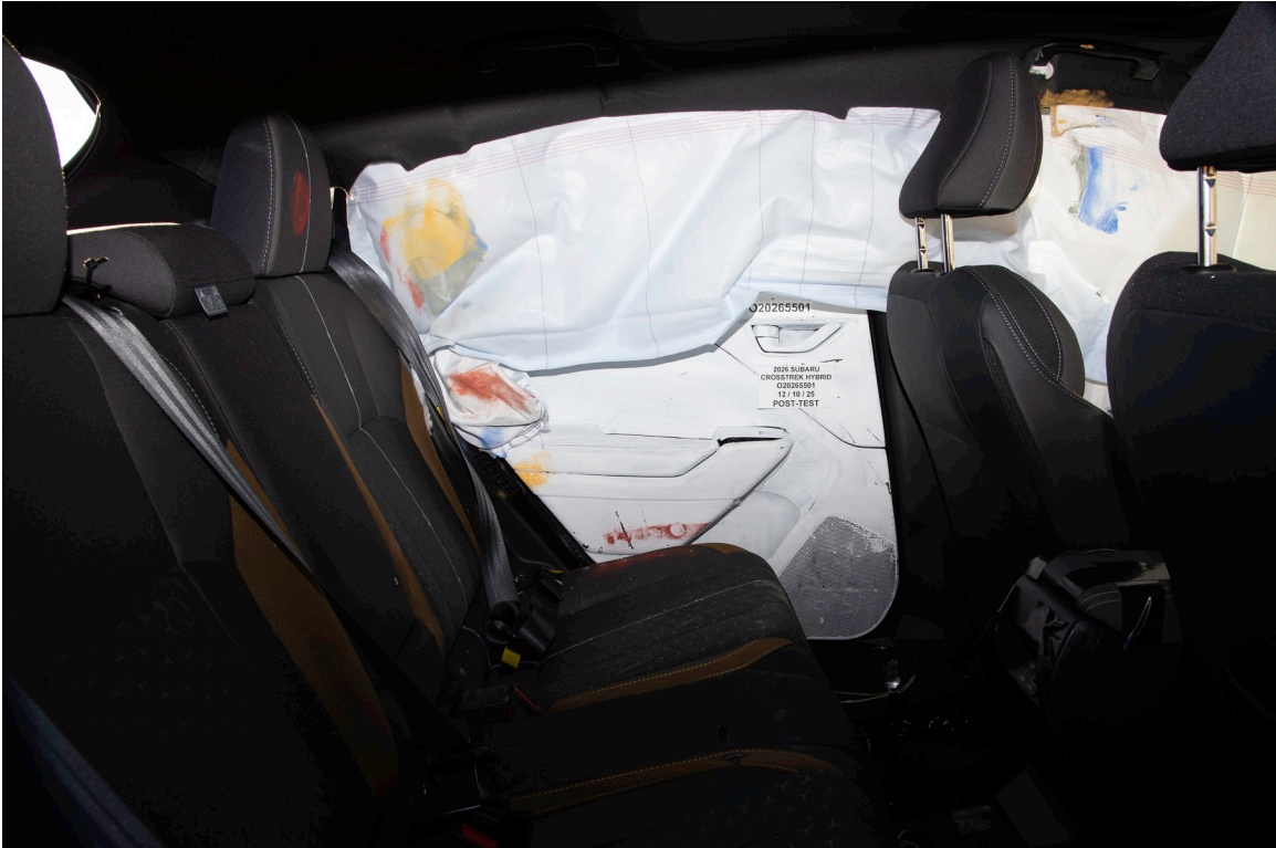
FIGURE 74. Post-Test Rear Passenger Inner Door Panel View
