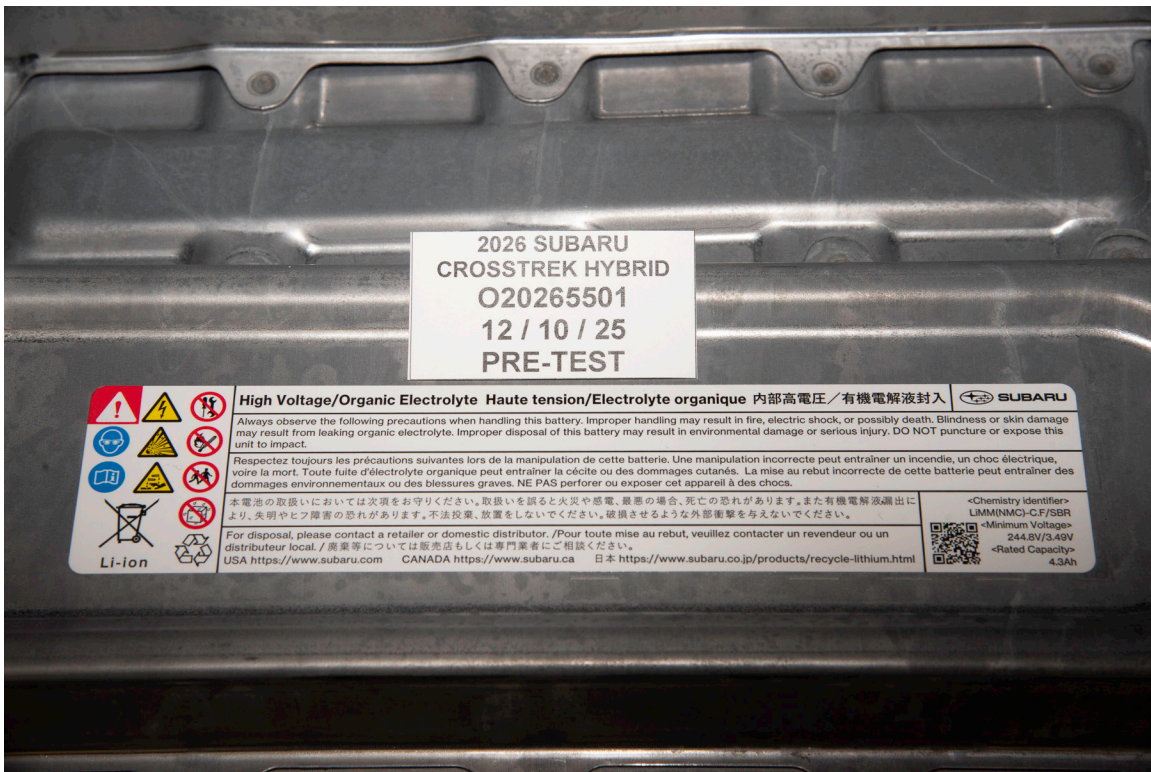
FIGURE 305-03. Other Vehicle Label(s) Related to Electrical Propulsion System
