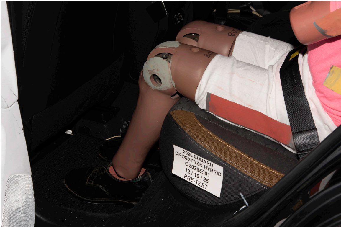
FIGURE 64. Pre-Test Placement of Rear Passenger Dummy's Feet
