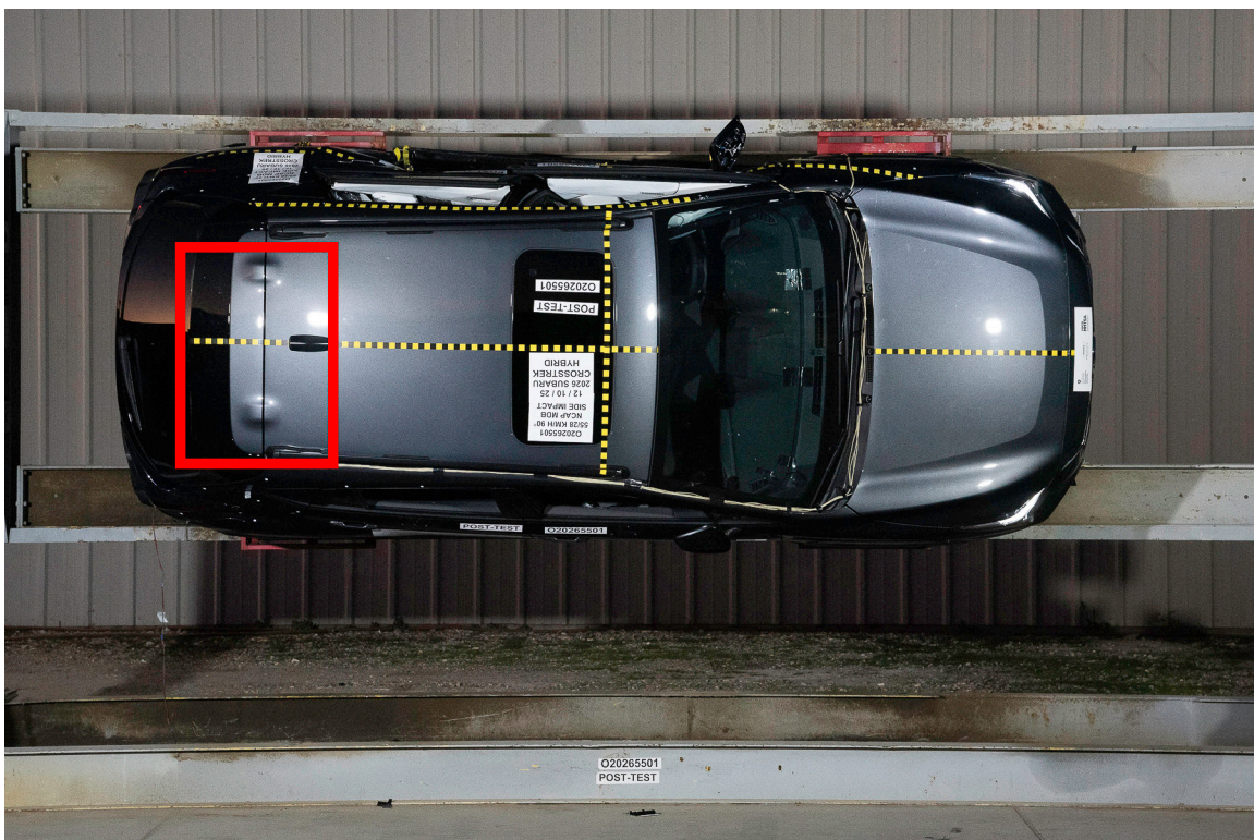
FIGURE 305-017. FMVSS No. 305 Static Rollover at 270°
