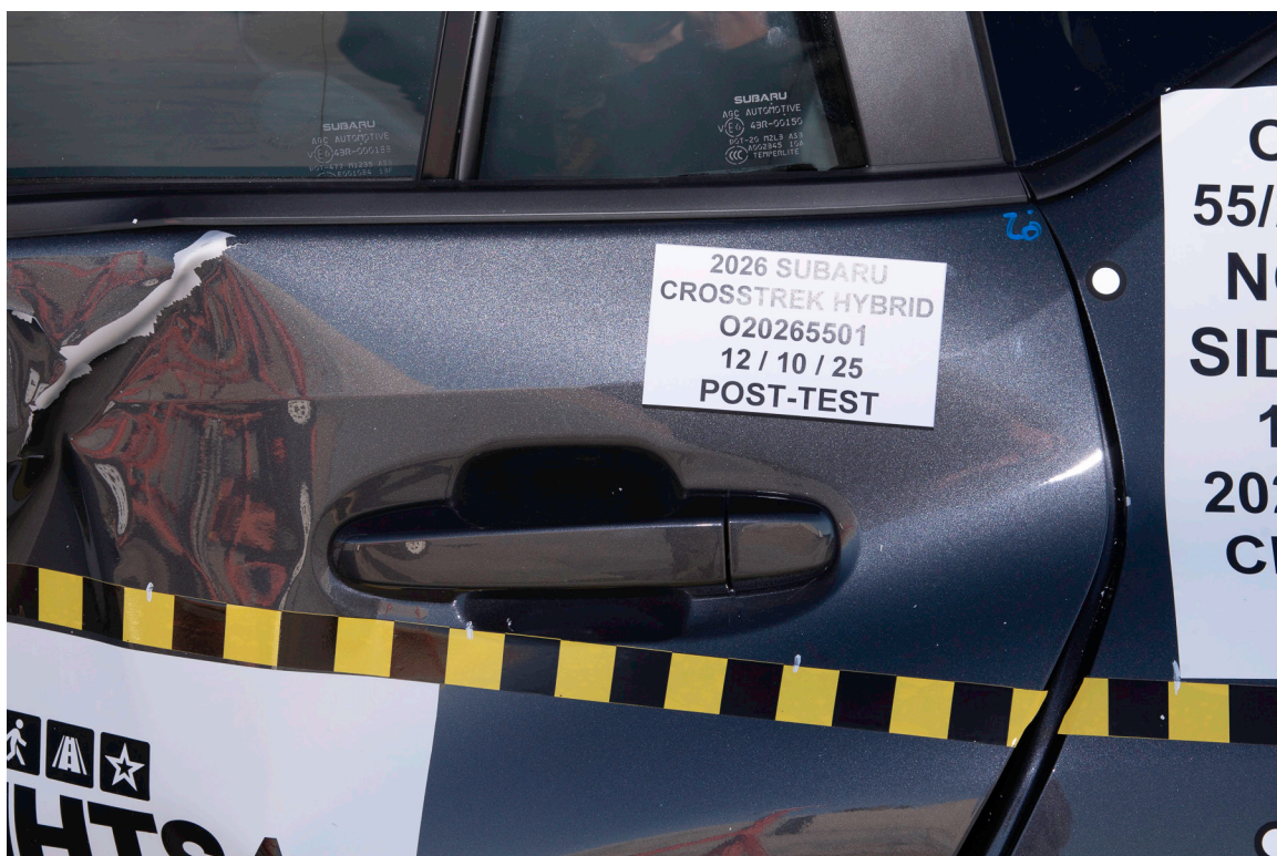
FIGURE 24. Post-Test Left Rear Door Latch Close-Up
