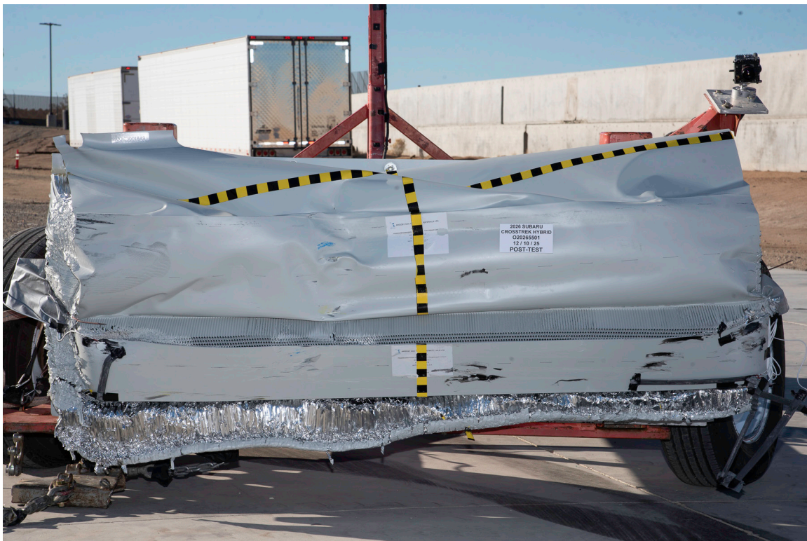
FIGURE 85. Post-Test Front View of MDB Impactor Face
