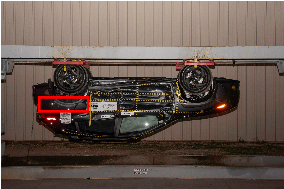
FIGURE 305-016. FMVSS No. 305 Static Rollover at 180°
